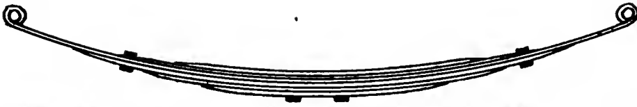
HEWITT CAR HALF-ELLIPTIC SPRING WITH THREE GRADED LEAVES BELOW THE MAIN LEAF AND TWO ABOVE.
